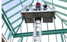
**SINGLE TOWER CONFIGURATION**Single tower shown with a 3M platform.
