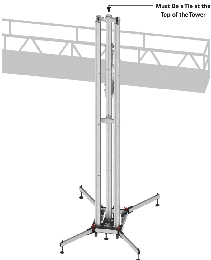
Figure 3.19 - Erecting the Freestanding System
